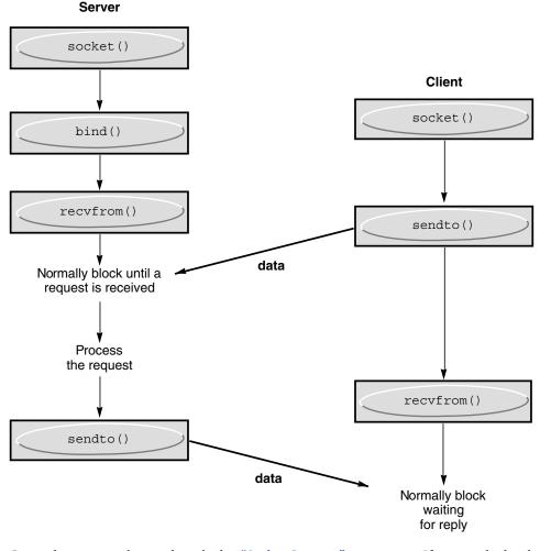
FIGURE 8-2 Connectionless Communication Using Datagram Sockets
