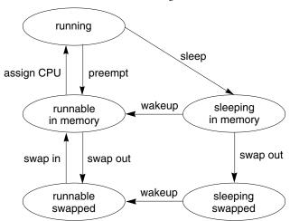
FIGURE 4-2 Process State Transition Diagram
