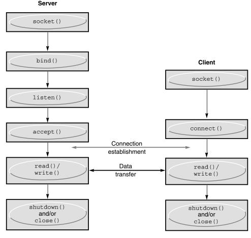
FIGURE 8-1 Connection-Oriented Communication Using Stream Sockets
