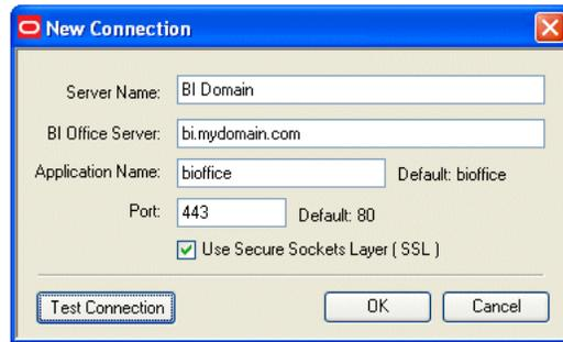
8. Click **Test Connection** to test the connection between the add-in and the Oracle BI EE Office Server.
