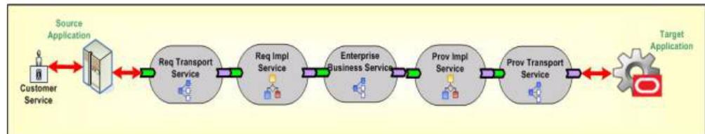
In the case of more complex situations in which the integration flow involves interactions with multiple applications, the requester application-specific AIA service presents its request to the mediator AIA service. The mediator AIA service triggers an AIA service that implements a workflow-like capability and manages all interactions with the provider application-specific AIA services through mediator AIA services.
