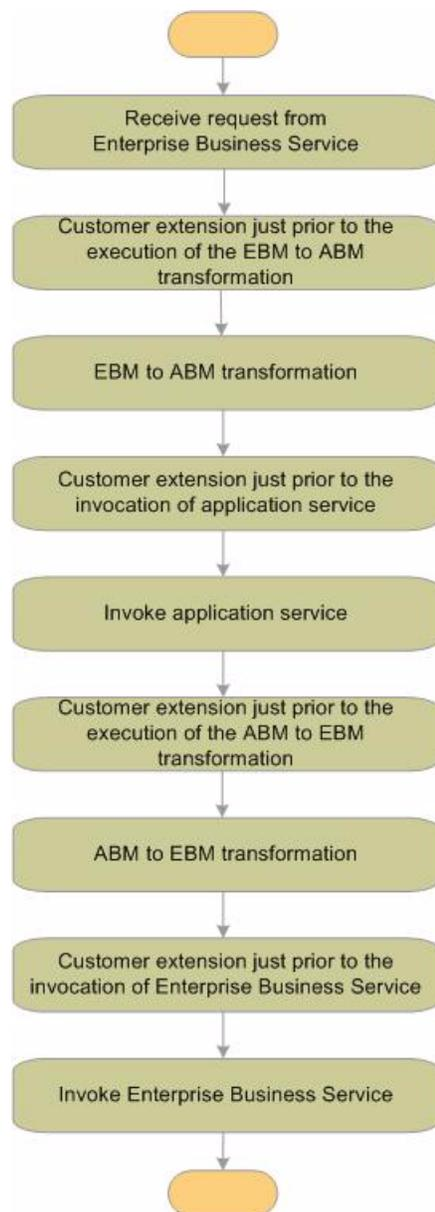
Figure 4–5 depicts the high-level flow of activities in a provider-specific ABCS. The diagram makes an assumption that the EBS with which it is interacting employs a fire-and-forget interaction style.
