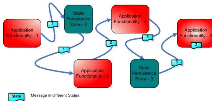
An integration flow represents the run-time path of a message. It is not a design-time artifact.
