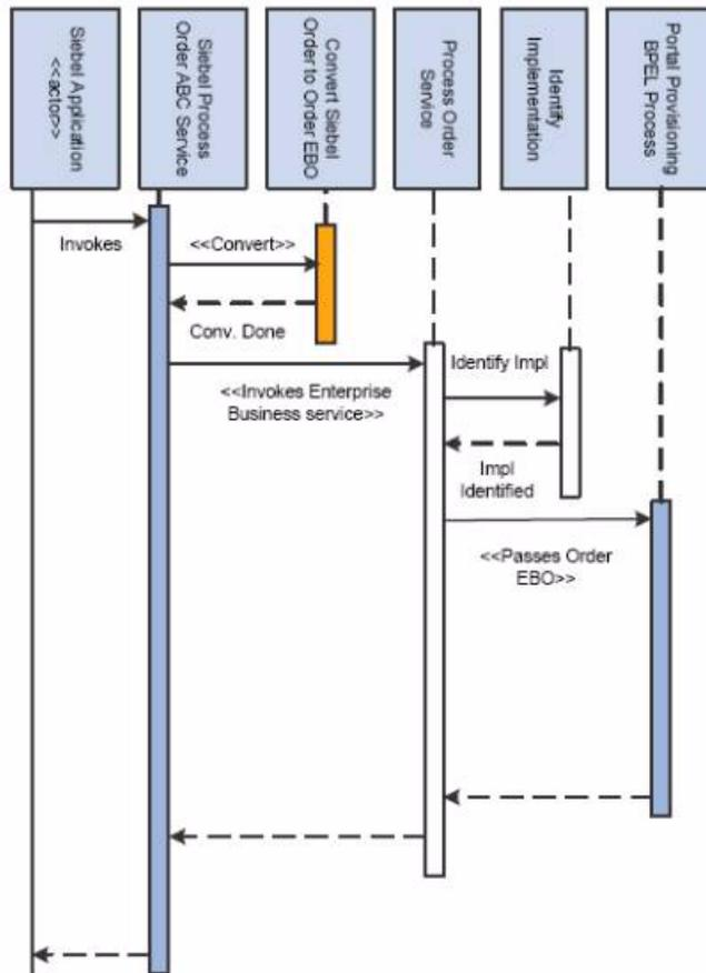
This diagram illustrates how to keep the BPEL processes application-independent.
