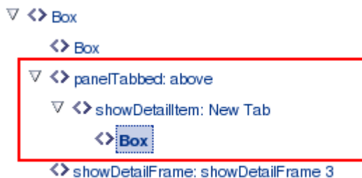
Figure 17–22 Tab Component in Source View
