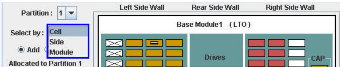
You can select by individual **Cell** (which includes drives), by module **Side**, or by complete **Module**.
