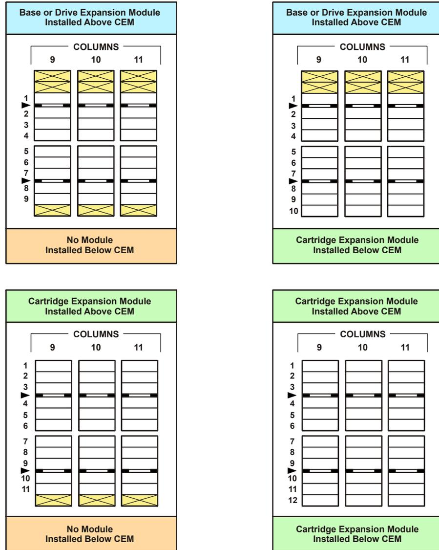
FIGURE A-7, shows a library with a Base Module that has eight reserved cells, one Drive Expansion Module, and one Cartridge Expansion Module.
