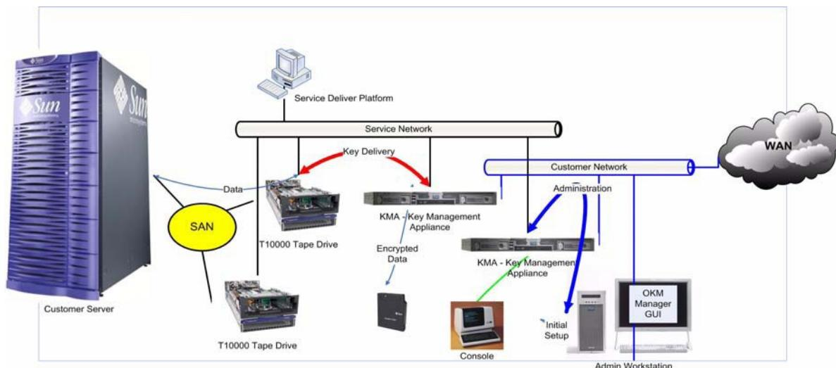
Figure 1-2. Typical Deployment of OKM Solution
