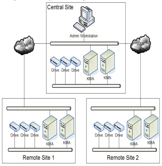
NOTE: Each KMA will have a second connection to the management network (not pictured above) for the ELOM interface used to perform initial configuration tasks.
