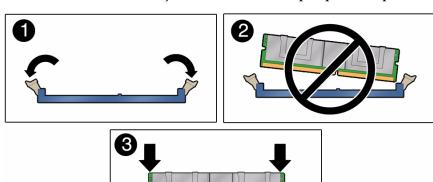
4. Line up the replacement DIMM with the connector.
