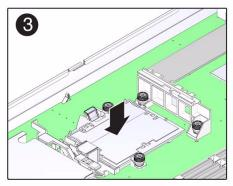
3. Seat the SP card into the connector by pressing the card toward the tabs while pressing down (panel 3).
