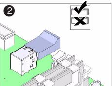
4. Plug your USB flash drive into the upper port of the USB connector (panels 1 and 2).
