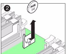
3. Install the replacement battery with the negative (-) side facing the nearby DIMM slot CMP0/BOB3/CH1/D0.
