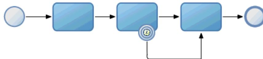
This diagram shows a BPMN process that contains an activity that has a deadline. If the token stays in the activity longer than the timer event specifies, then the timer event fires and the token moves to the next activity in the process.
