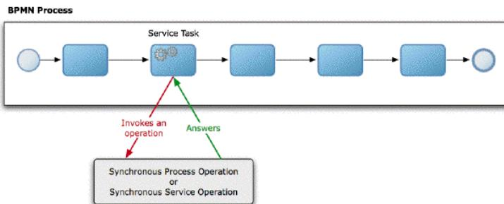
This figure shows a BPMN process that invokes a synchronous operation defined in an external service or in another BPMN process. This BPMN process uses message events to invoke the asynchronous operation.
