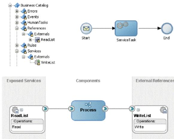
This Figure shows an SOA Composite that contains a file adapter with a read operation and another file adapter with a write operation. The file adapter with the read operation appears in the business catalog under the References predefined module, while the file adapter with the write operation appears under the Services predefined Module. The BPMN process contains a message start event that defines the interface using the ReadList interface and invokes the Write operation in the WriteList
