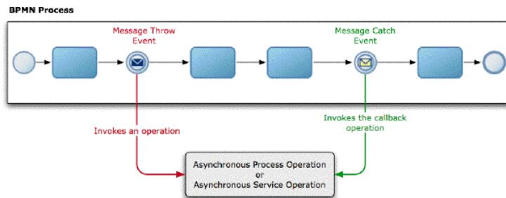
This figure shows a BPMN process that invokes an asynchronous operation defined in an external service or in another BPMN process. This BPMN process uses message events to invoke the asynchronous operation.
