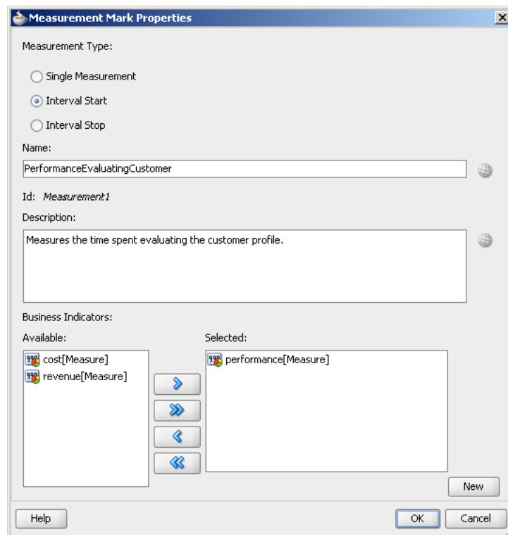
This figure shows the Measurement Mark Properties Dialog. This dialog enables you to configure the measurement mark type, provide a name and a description for the measurement mark, and select the business indicators to measure.
