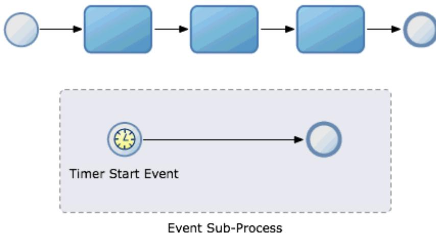
This diagram shows a process that contains a process deadline. If the token stays in the process longer than the timer start event in the event subprocess specifies, then the timer start event in the event subprocess fires. When the timer start event in the subprocess fires, the token moves to the event-sub process.
