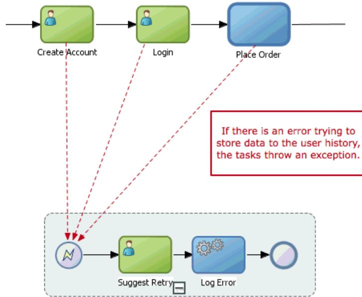
This figure three tasks that throw an exception when they are unable to write data to the user history. The process contains an event subprocess that handles the exceptions by suggesting the user to retry later and logging the error so that it is available for the system administrator to review it.
