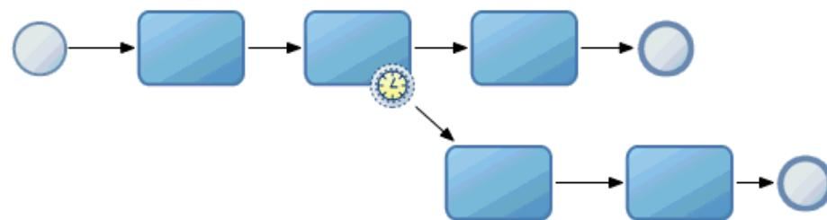
This diagram shows a process that contains an activity that runs additional activities while it is running. If the token is still in the activity when the non-interrupting timer event fires, then the BPMN Service Engine creates a copy of the token and routes it through the process flow the timer event defines.
