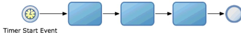
This diagram shows a process that starts with a timer event. The timer start event creates an token each time its time condition evaluates to true.
