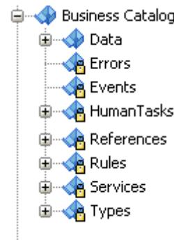
This figure shows the business catalog node of the Sales Quote example. The example contains a custom module named Data to store the components used in the project. The figure also shows the predefined modules Errors, Events, Human Tasks, References, Rules, Services and Types. These predefined modules are marked with a lock icon.
