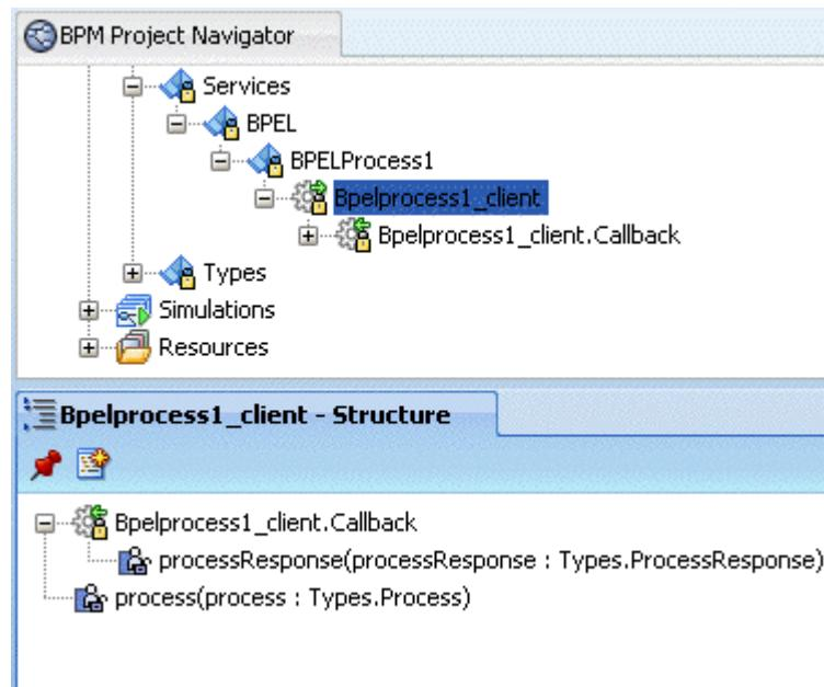
This figure shows the service component that represents an asynchronous BPEL process with a callback interface. The BPM Project Navigator displays the callback inner component under the service component. The Structure window displays the operations in the service component and the inner callback component. The inner callback component is expanded to view the list of operations it contains.
