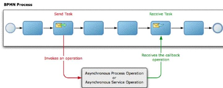
This figure shows a BPMN process that invokes an asynchronous operation defined in an external service or in another BPMN process. This BPMN process uses send and receive task to invoke the asynchronous operation
