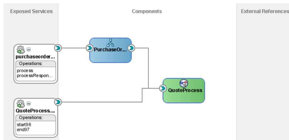
This SOA Composite diagram shows a BPEL process, Purchase Order, that uses the BPMN process Quote Process. The BPMN process is a partner link in the BPEL process.
