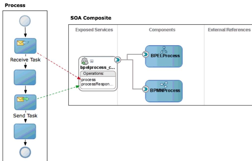
This figure shows a BPMN process defined using send and receive task that uses an interface from the business catalog. It also shows this reflects in the SOA Composite editor.
