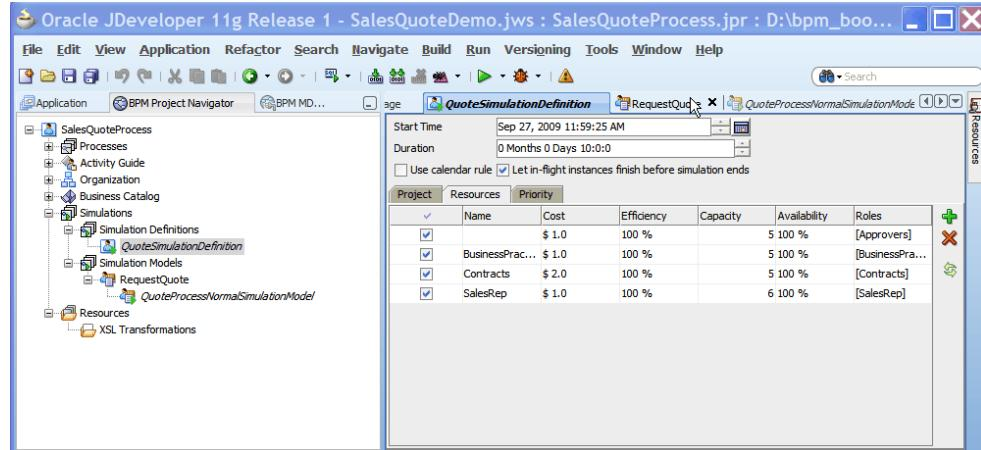
This graphic shows the BPM Project Navigator on the left. The simulation definition being configured is selected. On the right, the corresponding details page for that simulation definition is displayed. Within that details page, there are three tab pages: Project, Resources, and Priority. The Resources tab page is selected. The particular elements of both the details page and the Resources page are described in the surrounding text.
