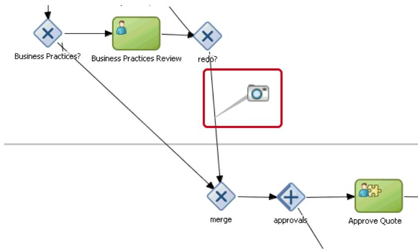
This image shows a single measurement mark placed on a transition between two exclusive gateways. This measurement mark stores the values of its associated business indicators have after the process instance completes the first exclusive gateway.
