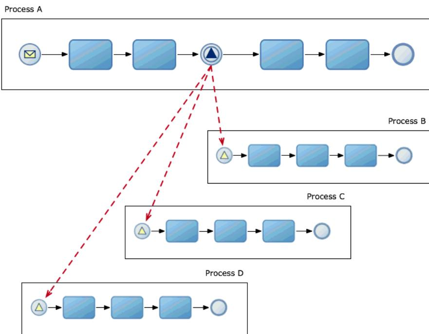
This figure shows a process A that broadcasts a signal. Processes B, C and D are configured to react to that signal.
