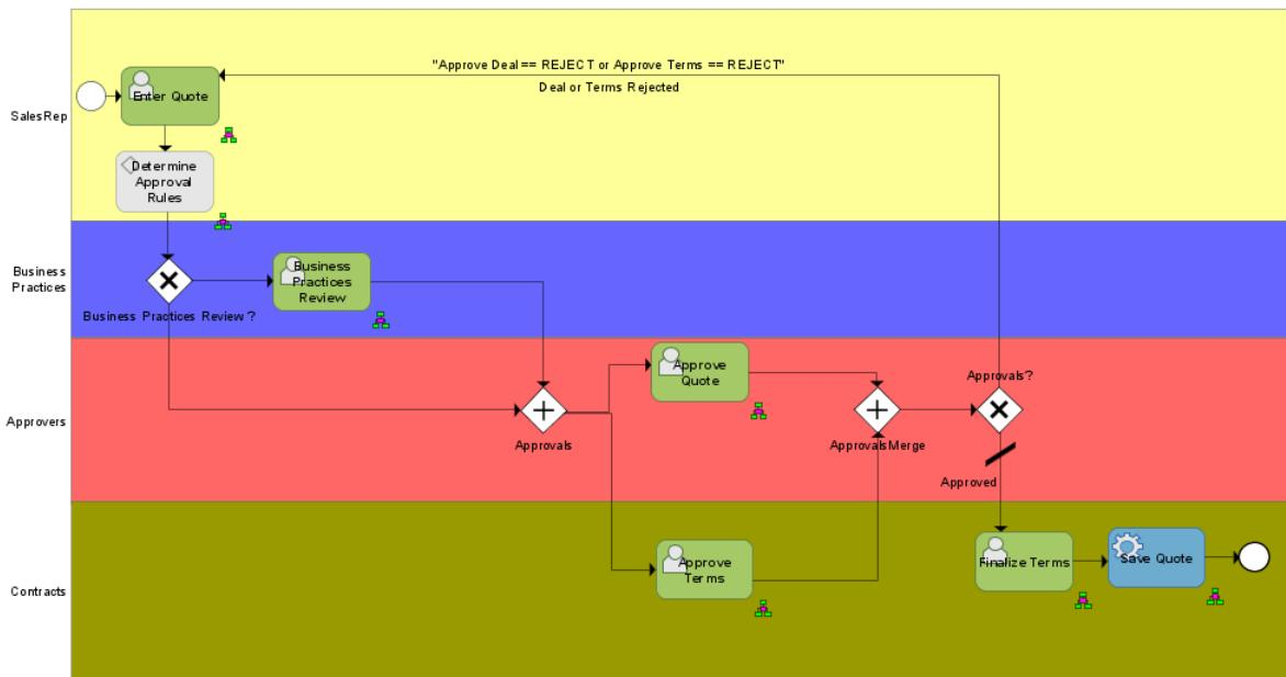
This figure shows a BPM Model of the Sales Quote example created using the BPA Architect application.
