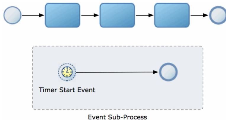
This diagram shows a process that runs activities in parallel to the main process flow. The timer start event in the event subprocess may fire multiple times while the process
