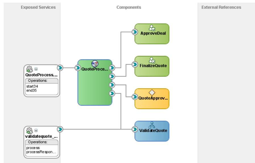
This SOA Composite diagram shows a BPMN process that uses Human Tasks, Business Rules and Service Adapters to implement its activities. Note that the BPMN process has a link to each of these SOA components.
