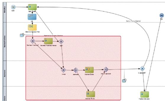
This image shows the portion of a process measured by a pair of interval measurement marks. Interval measurement marks measure the process business indicators in all the activities enclosed between the interval start and interval stop measurement marks.
