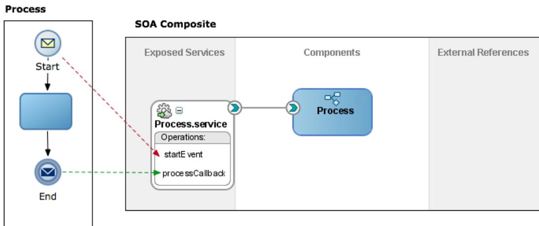
This figure shows a BPMN process that exposes a start operation and its corresponding callback, and how this reflects in the SOA Composite editor.
