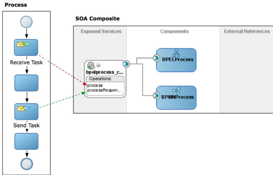
This figure shows a BPMN process that exposes an asynchronous operation defined using send and receive tasks, and how this reflects in the SOA Composite editor.
