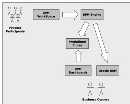
This diagram describes the cycle the process analytics data goes through. Process participants interact with the BPMN process using BPM WorkSpace. The BPMN Service Engine runs the activities in the BPMN process and stores the values of the business indicators in the process to BPM pre-defined cubes or Oracle BAM, or both. Business owners can monitor the process using Oracle BAM or BPM dashboards based on the pre-defined BPM cubes.
