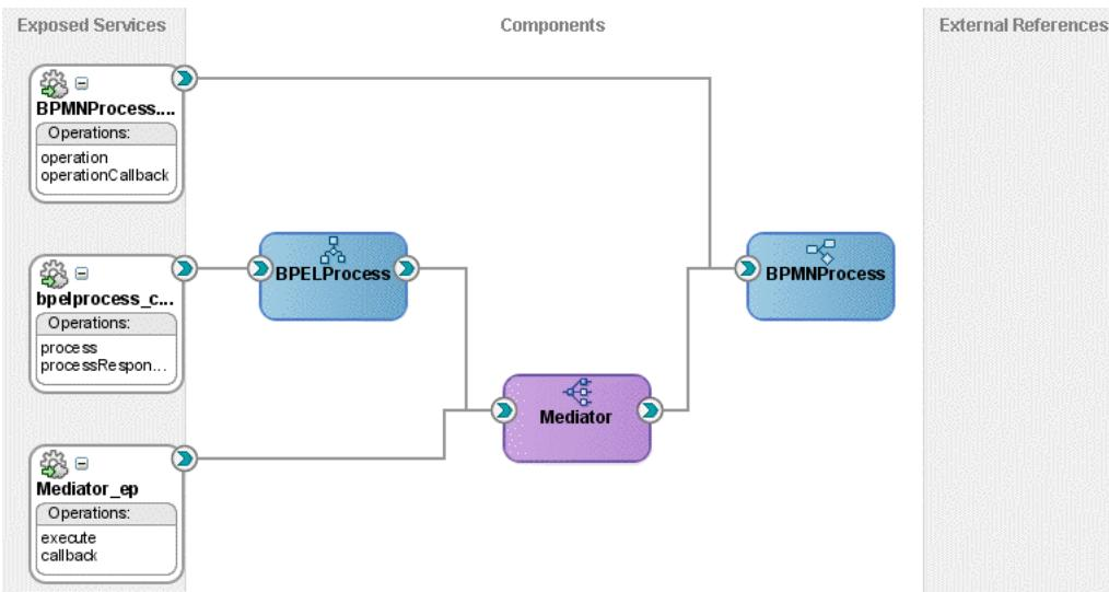
This figure shows a BPEL process that invokes a BPMN process through a Mediator.
