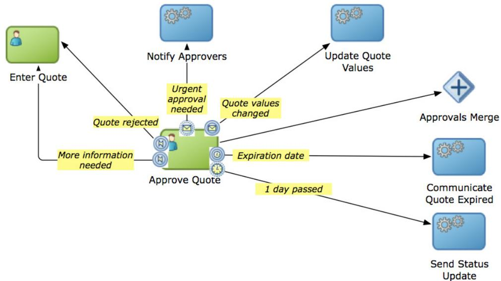
This figure shows the Approve Quote user task with different types of boundary events. The 'More information needed' and 'Quote rejected' error events and the 'Quote values changed' message events are interrupting boundary events. The 'Urgent approval needed' event is a non interrupting message event. The 'Expiration date' and '1 day passed' events are timer events.
