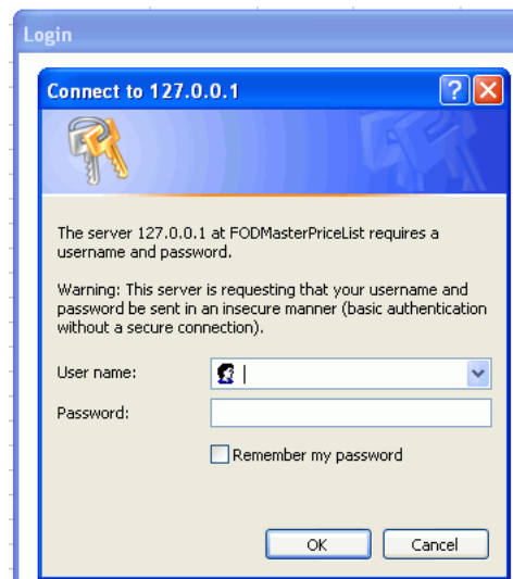
Figure 11-3 Dialog That Appears When a Fusion Web Application Uses Basic Authentication
