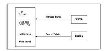
A C code harness performs the file handling (opening, closing and writing to files), and enables the PL/SQL and the formulas to interface.
