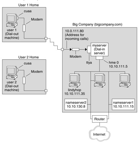
In this figure, a remote host dials out through its modem over telephone lines to Big Company's Intranet. Another host is configured to dial out to Big Company but currently is inactive. The calls from remote users are answered in the order received by the modem that is attached to the dial-in server at Big Company. A PPP connection is established between the peers. The dial-out machine can then remotely log in to a host machine on the Intranet.
