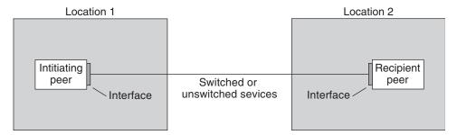
The previous figure shows a basic PPP link. The link has the following parts:
