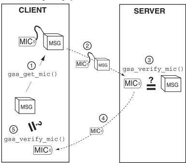
In the case of wrapped data, the gss\_unwrap() function never produces a separate MIC, so the recipient must generate it from the received and unwrapped message.
