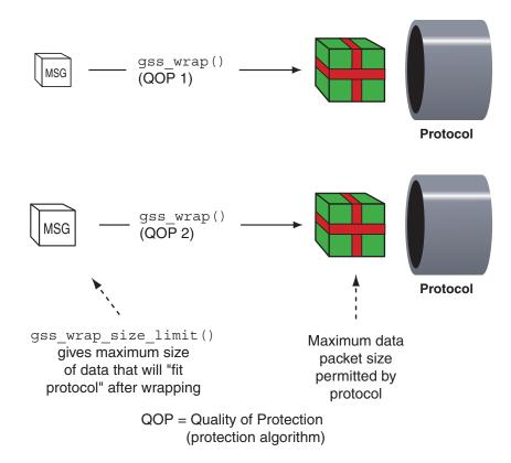
Regardless of whether confidentiality is applied, gss\_wrap() still increases the size of a message. gss\_wrap() embeds a MIC into the transmitted message. However, encrypting the message can further increase the size. The following figure shows this process.
