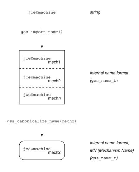
FIGURE 4–3 Internal Names and Mechanism Names
