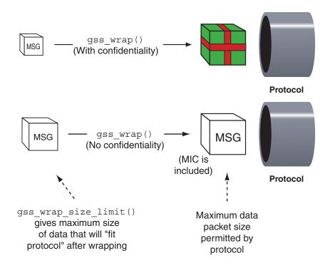
GSS\_S\_COMPLETE is returned if gss\_wrap\_size\_limit() completes successfully. If the specified QOP is not valid, GSS\_S\_BAD\_QOP is returned. "Wrapping and Sending a Message" on page 105 includes an example of how gss\_wrap\_size\_limit() can be used to return the maximum original message size.
