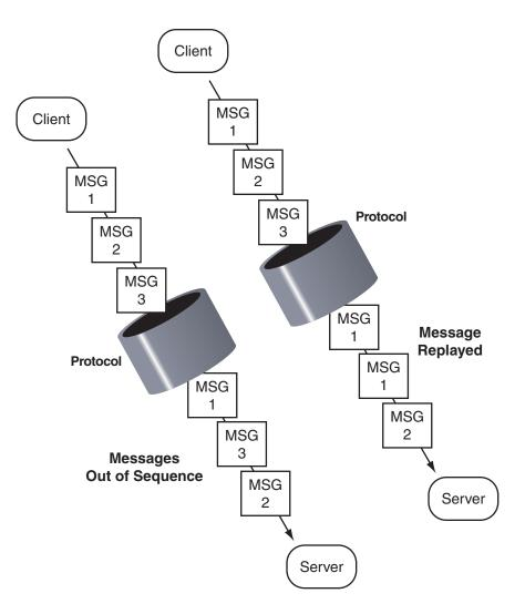
With  $gss_init_sec_context()$ , an initiator can check the sequence by applying logical OR to the *req\_flags* argument with either GSS\_C\_REPLAY\_FLAG or GSS\_C\_SEQUENCE\_FLAG.
