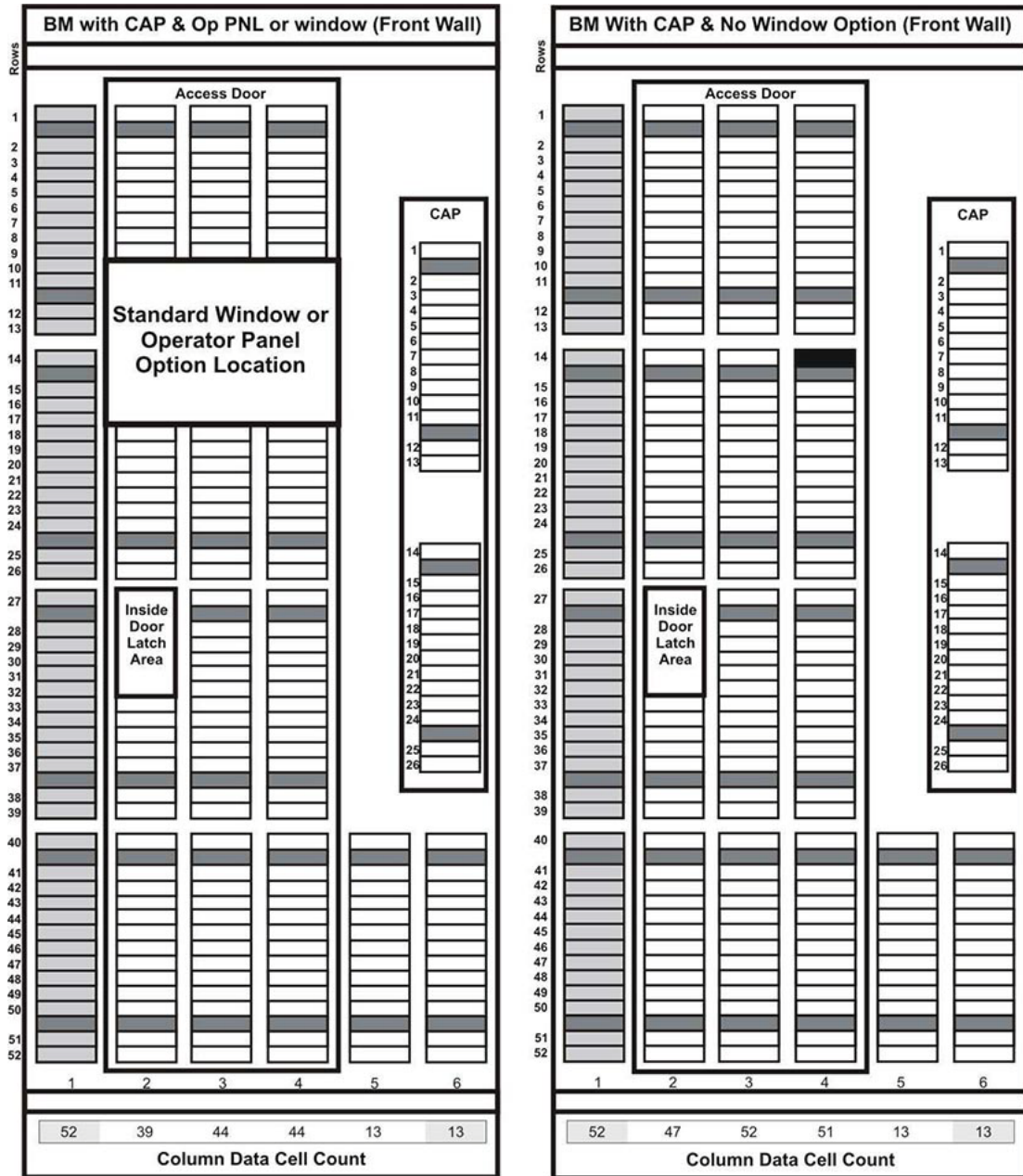
Figure E-13 Base Module, Front Wall
