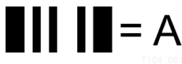
Figure F-1 Code 39 Barcode Standard — Letter A
