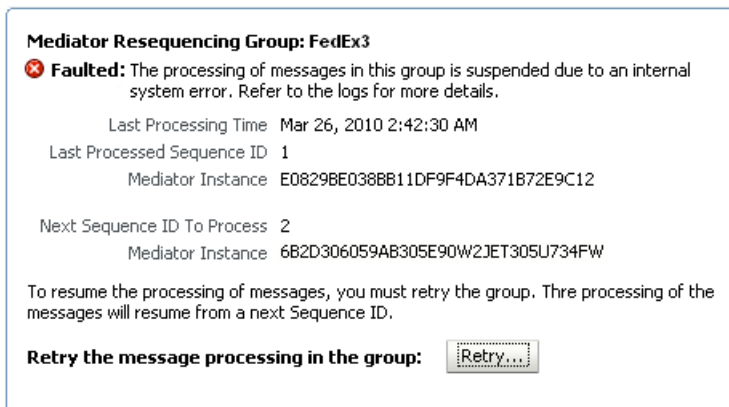
Figure 17–8 Group Is Faulted Due to a System Error
