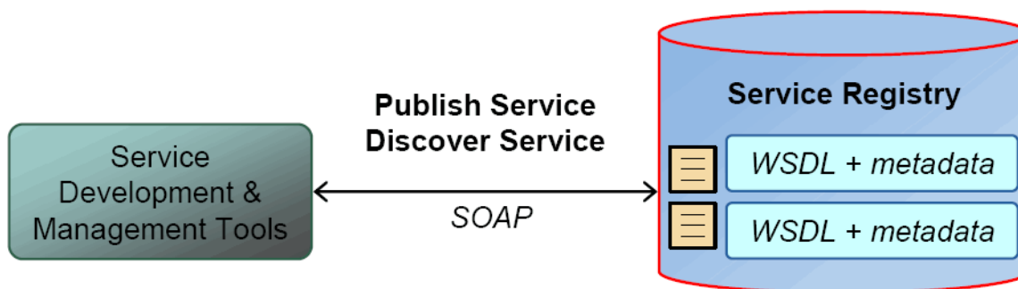
Figure 1–11 Service Publishing and Discovery with UDDI
