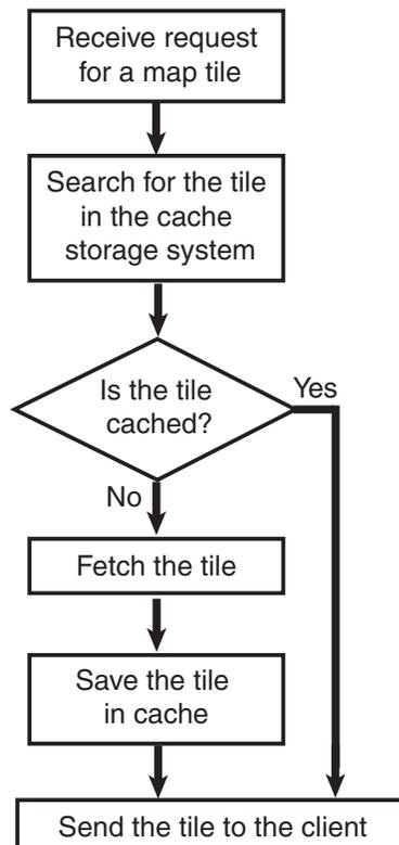
As shown in [Figure 8-4](#), when the map tile server receives a request for a map tile, it searches for the tile in the cache storage system. If the tile is cached, the map tile server sends the tile to the client. If the tile is not cached, the map tile server fetches the tile, saves in the cache, and sends it to the client.
