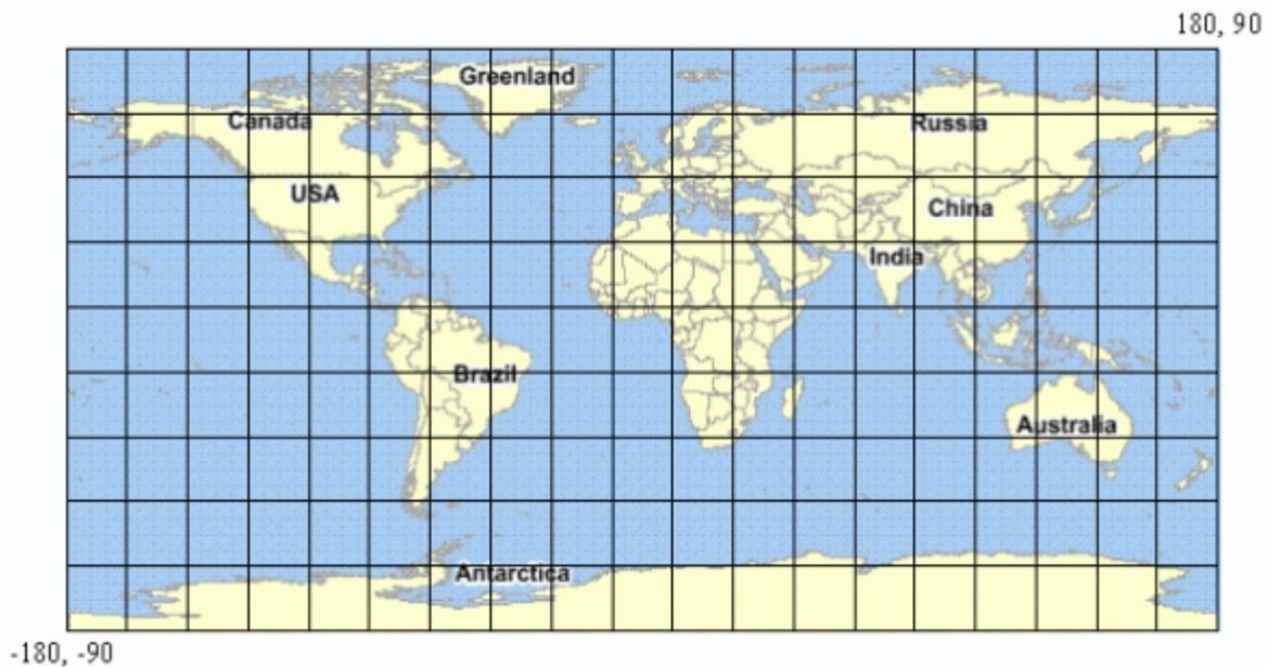
On each zoom level, the map tiles are created by equally dividing the whole map coordinate system along the two dimensions (X and Y, which in [Figure 8–5](#) represent latitude and longitude). The map tile server needs this dimensional information of the map coordinate system in order to create map image tiles, and therefore you must include this information in the map tile layer configuration settings.
