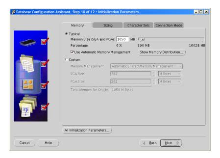
This window provides different database parameters. You can navigate to the settings of memory, character sets, database sizing, and connection mode. Usually all parameters are set by the selected template and you don't need to change them, but experienced users can modify some parameters depending on the database size and number of users.
