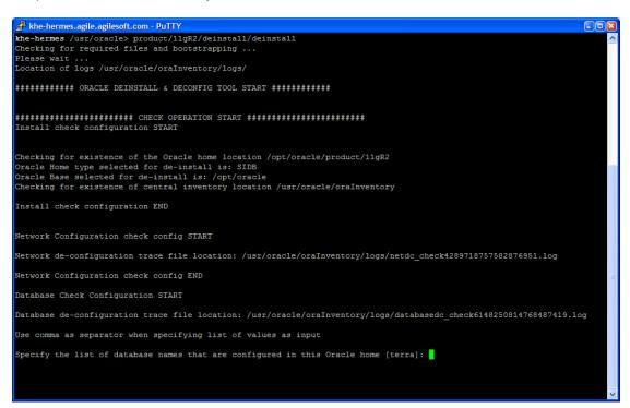
Specify all single instance listeners that are to be deconfigured as well as database names that are configured in this Oracle home. Finally, confirm the deinstallation with 'y'.
