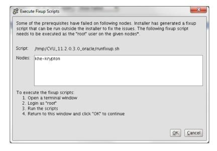
**Note** Using the fixup scripts does not ensure that all the prerequisites for installing the Oracle database are satisfied. You must still verify that all the pre-installation requirements are met to ensure a successful installation.
