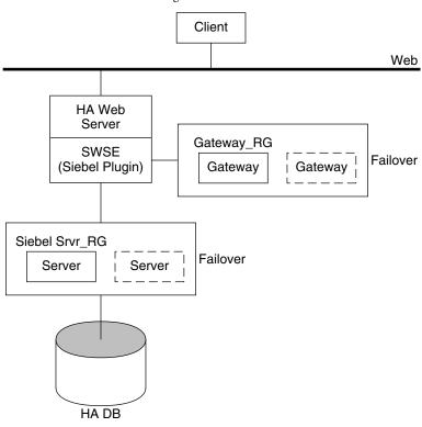
FIGURE 1-1 Standard Siebel Configuration
