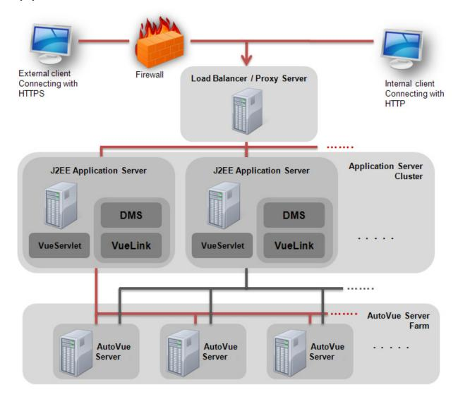
Most document management systems are designed as J2EE Web applications and can be deployed into a wide range of J2EE application servers. When setting up a cluster of application servers, a load balancer is the main entry point for all communications. When accessing the DMS from a Web browser, the request is dispatched by the load balancer to one of the application servers. If your DMS is deployed in a clustered environment, ensure that it works reliably in the clustered environment.
