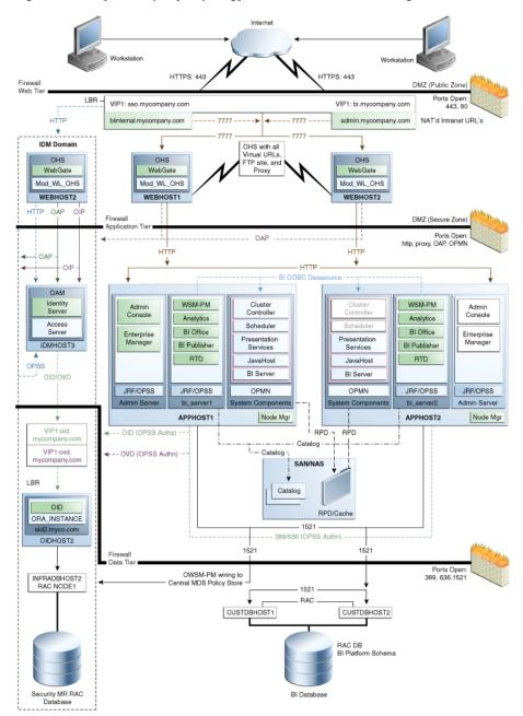
Figure 2–1 MyBICompany Topology with Oracle Access Manager
