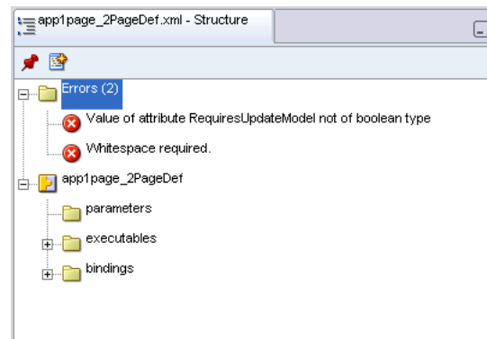
Figure 31–1 The Structure Window Displays XML Errors
