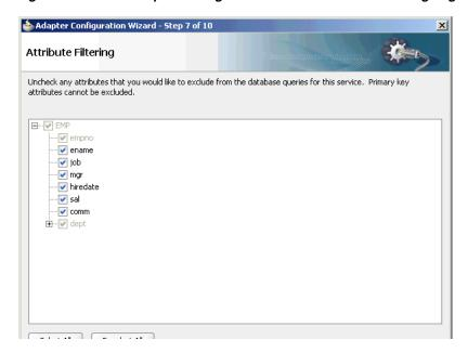
Figure 9-16 The Adapter Configuration Wizard: Attribute Filtering Page
