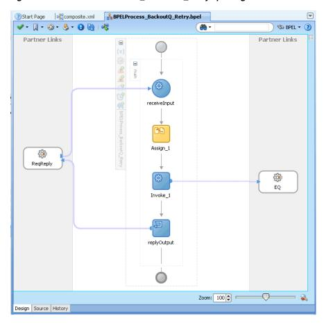
Figure 10–93 The BPELProcess\_BackoutQ\_Retry.bpel Page
