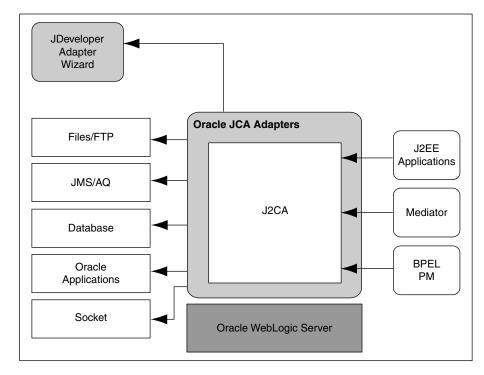
Figure 1–2 Oracle Technology Adapters Architecture
