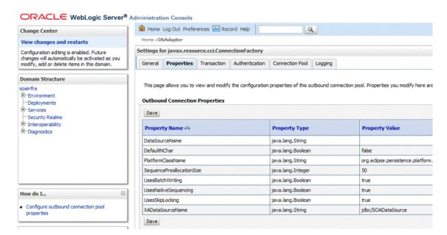
Figure 9–30 Database Adapter Properties in the Oracle WebLogic Administration Console
