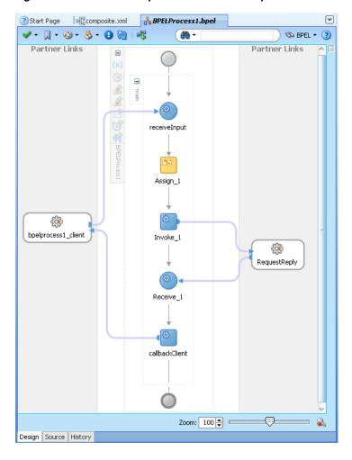
Figure 7-32 The JDeveloper - BPELProcess1.bpel
