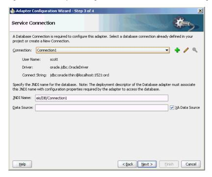
Figure 9–7 The Adapter Configuration Wizard: Service Connection Page
