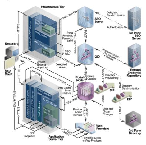
Figure 1–5 Communication Flow and Protocols
