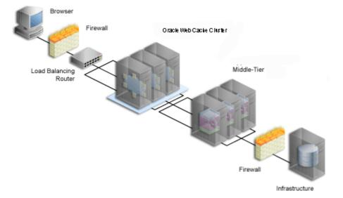
Figure 1–6 Adding Oracle Web Cache to a Medium to Large Portal Configuration
