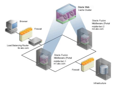
Figure 6–1 Multiple Middle-Tier Configuration with a Load Balancing Router
