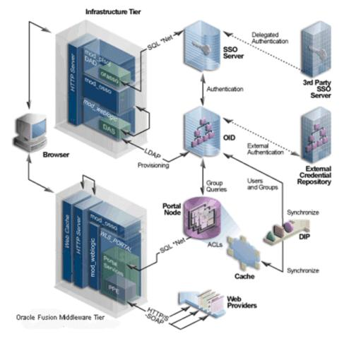
Figure 7–1 Oracle Portal Security Architecture
