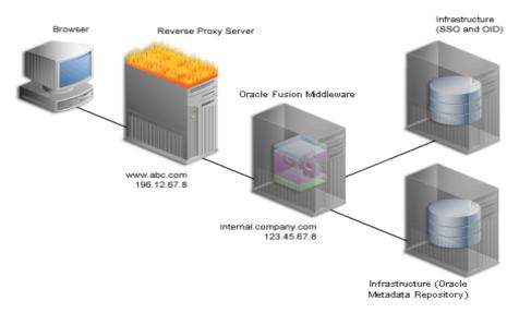
Figure 6–5 Reverse Proxy Server Configuration
