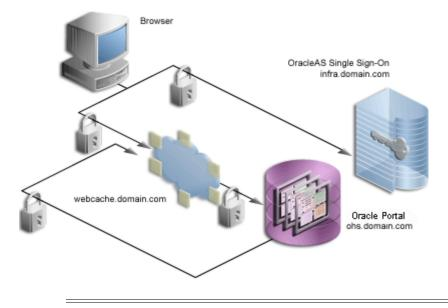
Figure 7–21 Secured Connections Throughout the System
