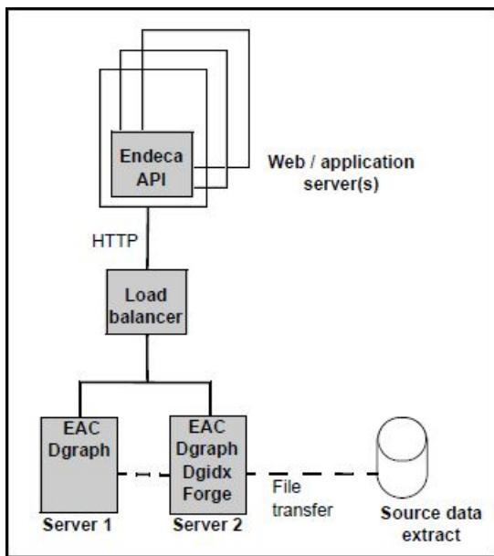
The advantage of this scenario is low cost and MDEX Engine redundancy. If one MDEX Engine is offline for any reason, the load balancer distributes user queries to the other MDEX Engine.
