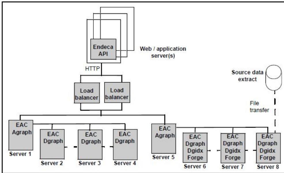
There are several advantages of this scenario. First, the cluster of MDEX Engines is redundant and one cluster of MDEX Engines runs on dedicated servers, so those servers do not need to share resources for Forge processing and indexing. Second, this scenario employs two load balancers to reduce potential offline time if one balancer fails.
