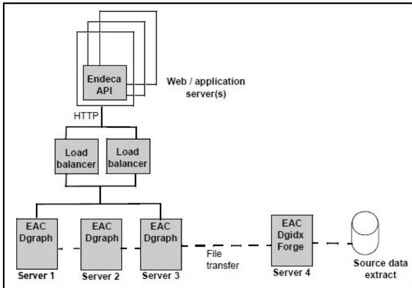
The advantage of this scenario is that overall throughput and redundancy is high. Each MDEX Engine runs on a dedicated server, so the servers do not need to share resources for Forge processing and indexing. Also, this scenario employs two load balancers to reduce potential offline time if one balancer fails.
