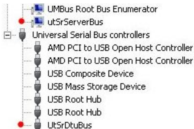
Figure 17.8 Verifying USB Redirection in Windows Device Manager
