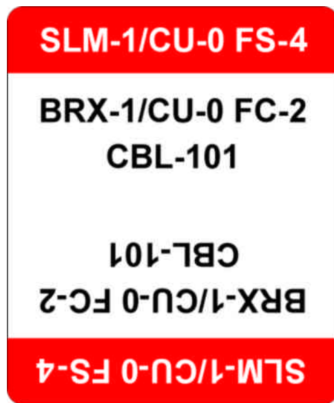
Figure 2 FC cable label sample
