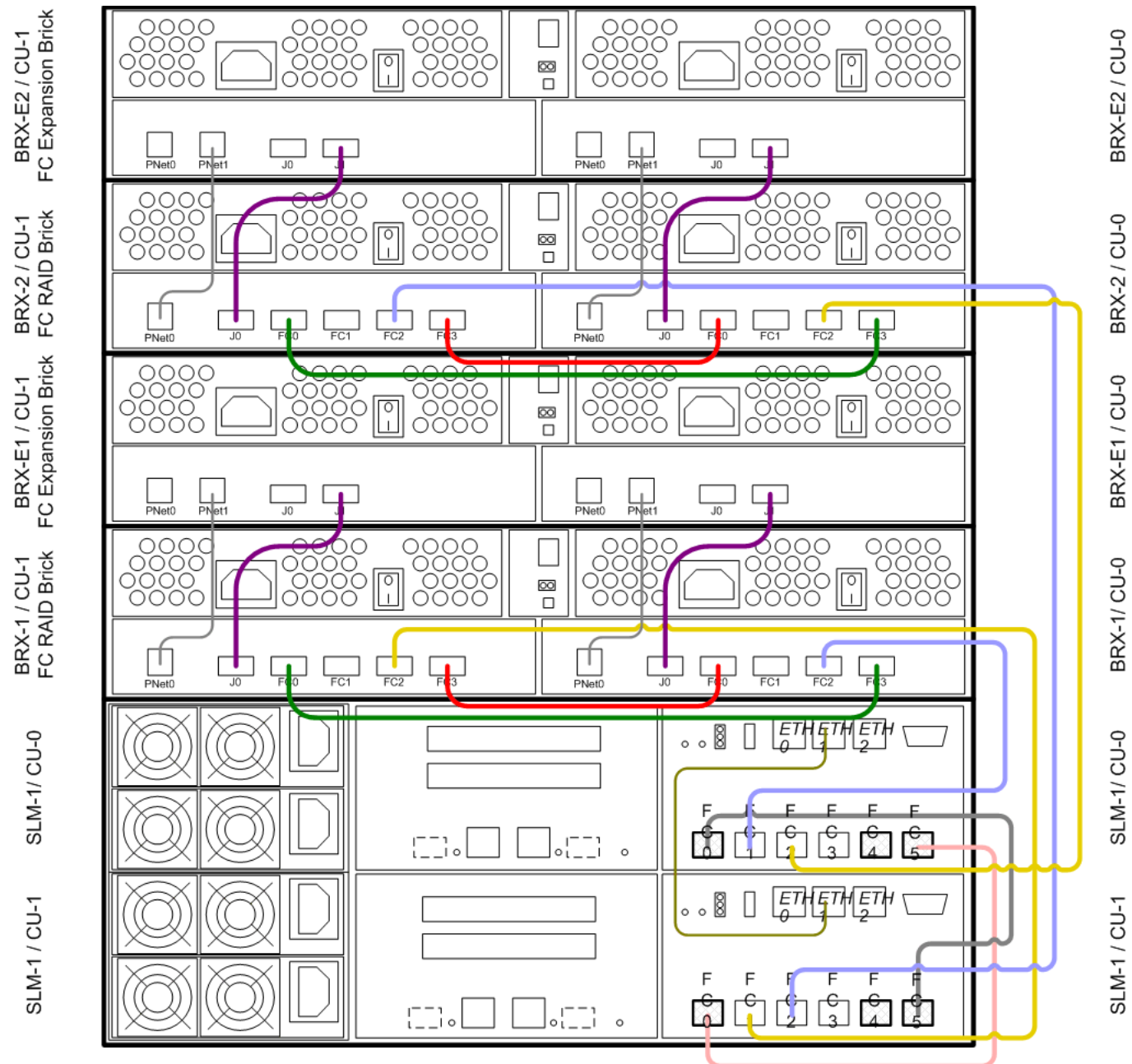
Figure 6 Sample cabling for a 1x4 Pillar Axiom 300 system (FC Bricks)
