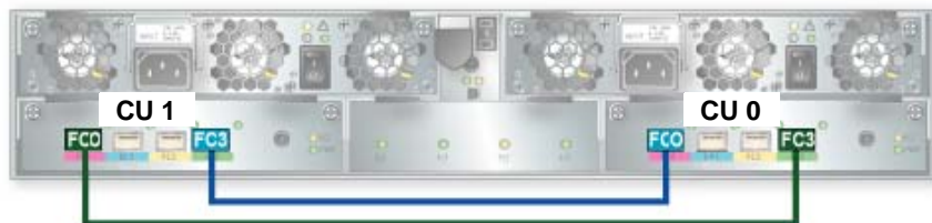
Figure 33 FC cables connect Brick RAID controllers for failover
