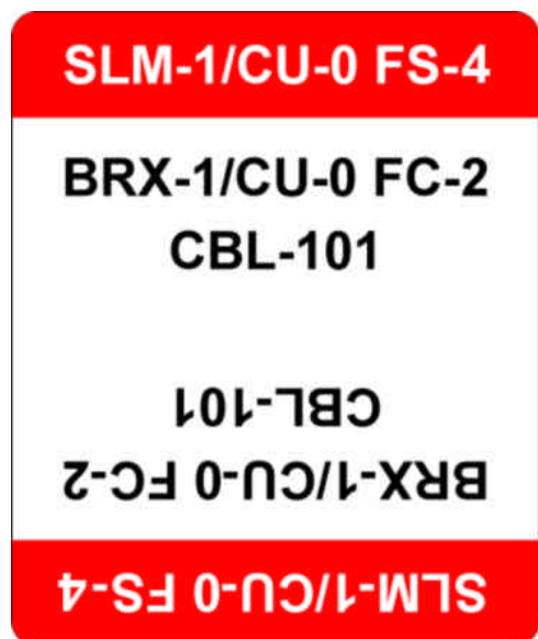
Figure 2 FC cable label sample
