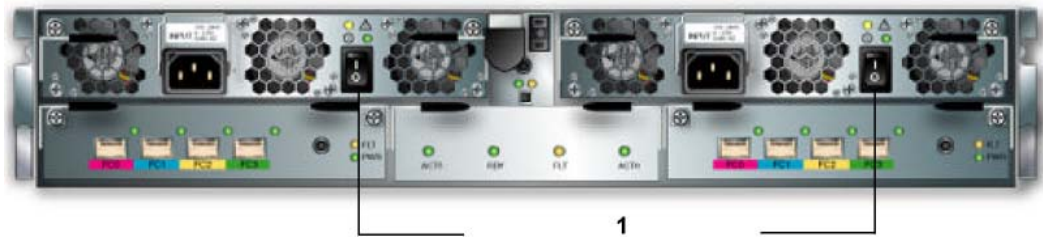
Figure 42 Turn on Brick power
