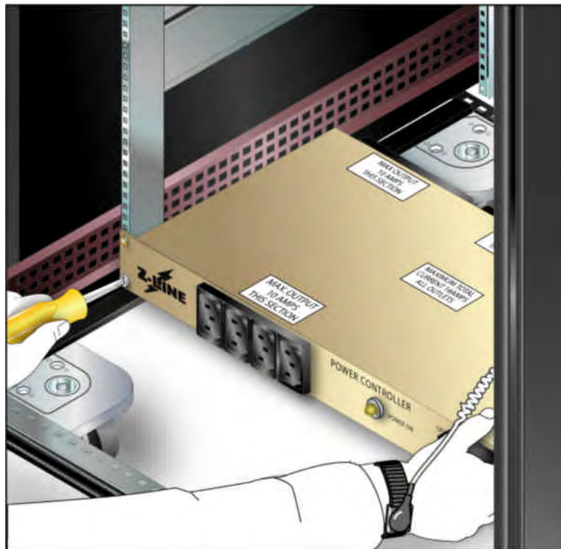
Figure 25 Securing a 1U PDU in the bottom of a rack
