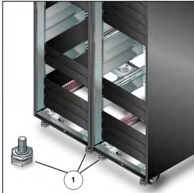
Figure 6 Adjacent anchor bolts at the front of the racks
