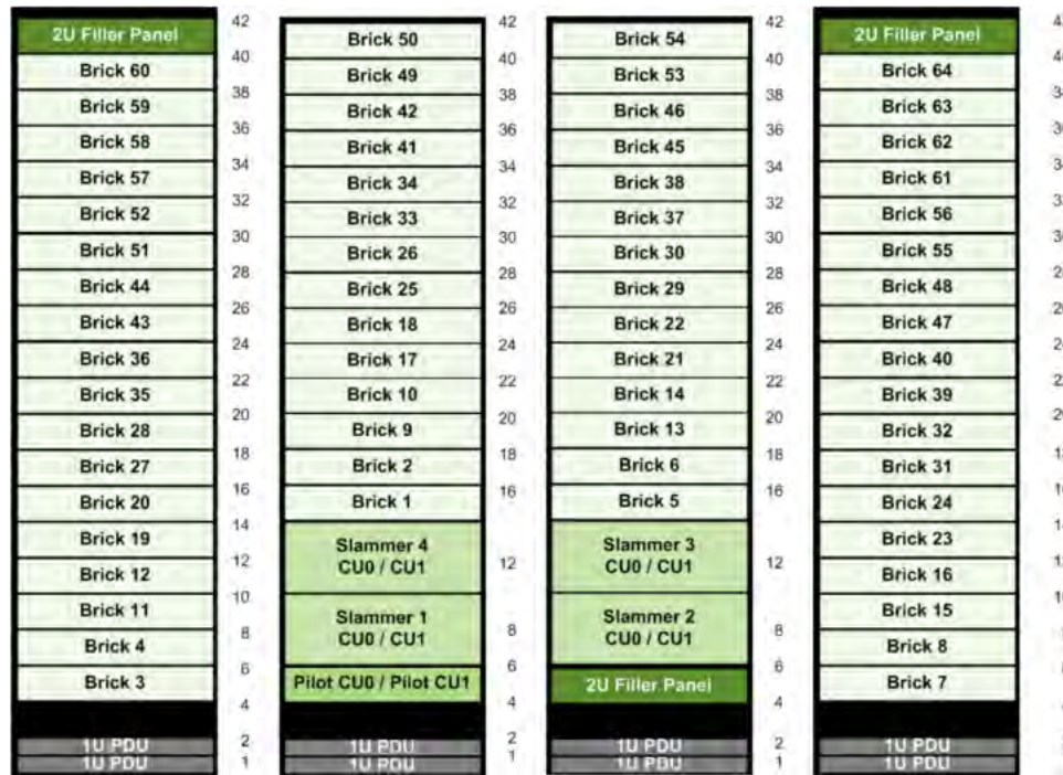
Figure 16 Fully loaded 42U racks for four Slammers and 64 Bricks
