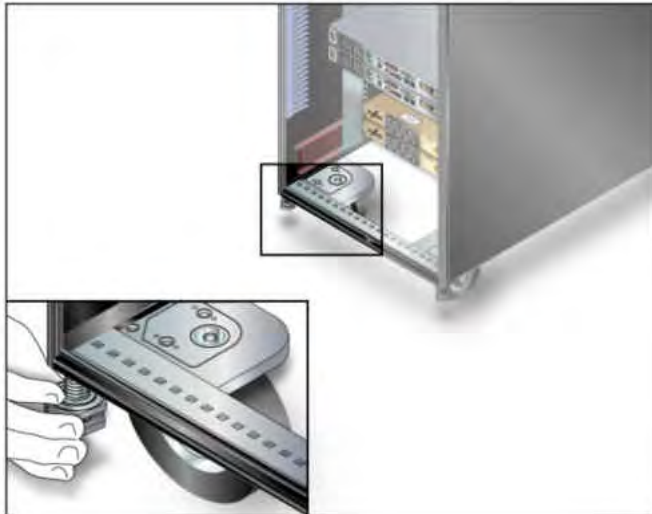
Figure 9 Attach anchor bolts to rack
