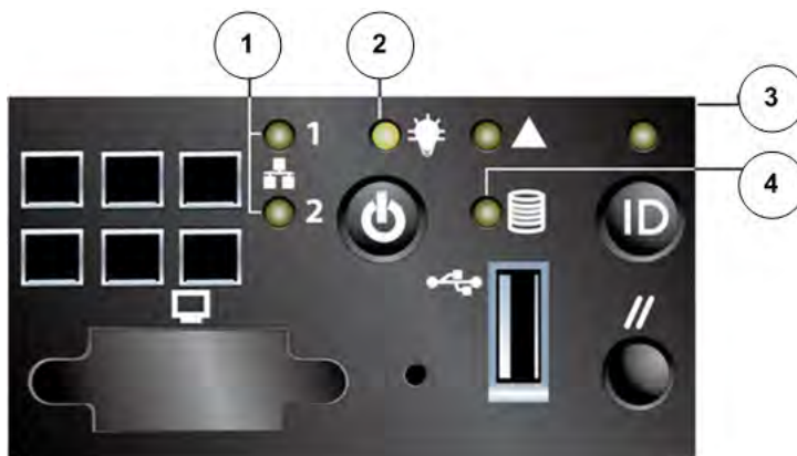
Figure 9 LEDs on a Pilot CU (1450-00164-XX) Intel, front panel
