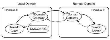
In the example, you must also create a DMCONFIG file for Domain Y that complements the DMCONFIG file created for Domain X. That is, a local domain access point in the Domain X DMCONFIG file would be a remote domain access point in the Domain Y DMCONFIG file, and a remote domain access point in the Domain X DMCONFIG file would be a local domain access point in the Domain Y DMCONFIG file. The example demonstrates the use of the TDomain gateway server.
