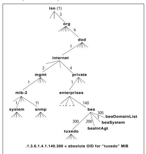
Figure 1-2 SNMP MIB Object Identifier Hierarchy and Format
