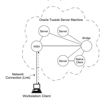
Figure 1-1 Oracle Tuxedo ATMI Workstation Component Operation
