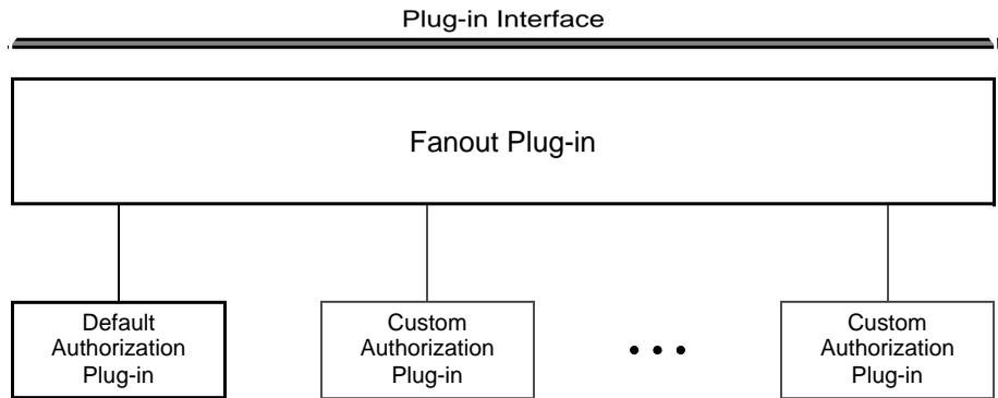
The default authorization implementation consists of a fanout plug-in and a default authorization plug-in. A custom implementation consists of the fanout plug-in, the default authorization plug-in, and one or more custom authorization plug-ins.
