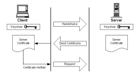
After the client verifies the certificate from the server, the client and server can now communicate securely using encrypted keys known only to the client and server.
