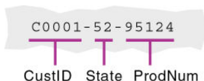
Figure 5 Transforming a Product Code Stored in a PRODID Column
