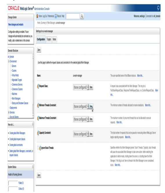
Step 8: Click on New button to create Minimum Threads Constraint
