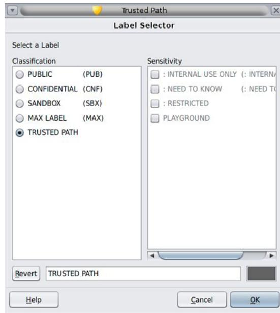
The label builder GUI in the figure includes the Classification and Sensitivity lists, the default label, and the Revert, Help, Cancel, and OK buttons.
