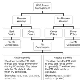
The driver can implement one of the two power management schemes described at the bottom of [Figure 20-5](#). The passive scheme is simpler than the active scheme because the passive scheme does not do power management during device transfers.
