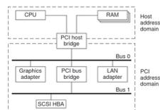
The PCI host bridge provides an interconnect between the processor and peripheral components. Through the PCI host bridge, the processor can directly access main memory independent of other PCI bus masters. For example, while the CPU is fetching data from the
