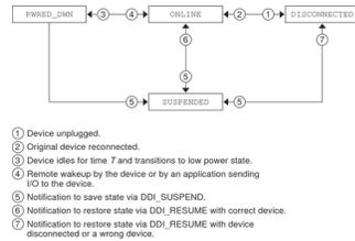
This state machine and its four states can be augmented with driver-specific states. Device states `0x80` to `0xff` can be defined and used only by client drivers.
