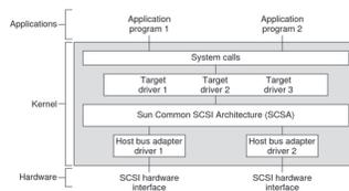
The lower-level software component consists of a SCSA interface layer and one or more host bus adapter drivers. The target driver is responsible for the generation of the proper SCSI commands required to execute the desired function and for processing the results.
