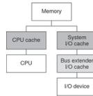
When an attempt is made to read data from main memory, the associated cache checks for the requested data. If the data is available, the cache supplies the data quickly. If the cache does not have the data, the cache retrieves the data from main memory. The cache then passes the data on to the requester and saves the data in case of a subsequent request.
