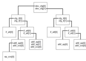
The `dev_cfg` array shown in the above figure contains nodes that correspond to configurations. Each node contains the following information:
