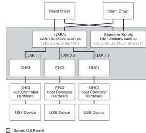
Figure 20-2 shows interfaces in more detail than Figure 20-1 does. Figure 20-2 shows that the USBA is a kernel subsystem into which a client driver can call, just as a client driver can call DDI functions.
