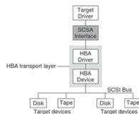
The *HBA transport layer* is a software and hardware layer that is responsible for transporting a SCSI command to a SCSI target device. The HBA driver provides resource allocation, DMA management, and transport services in response to requests made by SCSI target drivers through SCSA. The host adapter driver also manages the host adapter hardware and the SCSI
