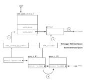
The walker is designed to iterate over the list of proc\_t structures in the kernel. The head of the list is stored in the global practive variable, and each element's p\_next pointer points to the next proc\_t in the list. The list is terminated with a NULL pointer. In the walker's init routine, the practive symbol is located using mdb\_lookup\_by\_name step (1), and its value is copied into the mdb\_walk\_state\_t pointed to by wsp.
