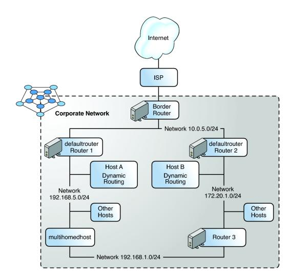
FIGURE 3-1 Autonomous System With Multiple IPv4 Routers
