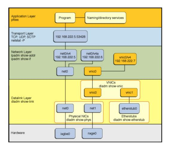
FIGURE 1-1 Oracle Solaris 11 Network Protocol Stack
