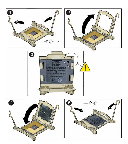
b. Hold the processor ILM assembly load plate open with one hand and position the processor socket cover over the top of the load plate so that 1) the arrow on the processor socket cover is aligned with the arrow on the load plate and 2) the fasteners on one side of the cover (the fasteners are located on the underside of the cover) are inside the load plate (it does not matter which side), and use your thumb to press the other side of the processor socket cover into the load plate. [3].
