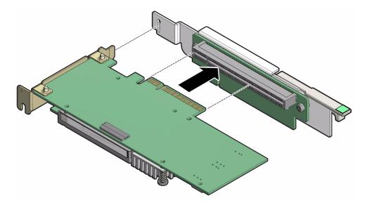
4. Install the PCIe riser into the server.
