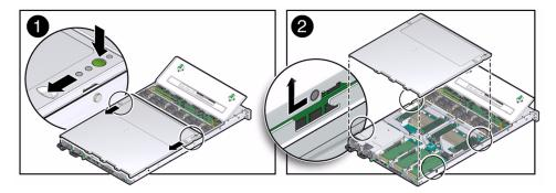
4. Lift the cover off the chassis and set it aside [2].
