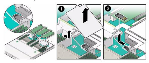
3. Grasp the USB flash drive and pull it out of the internal USB port [2].
