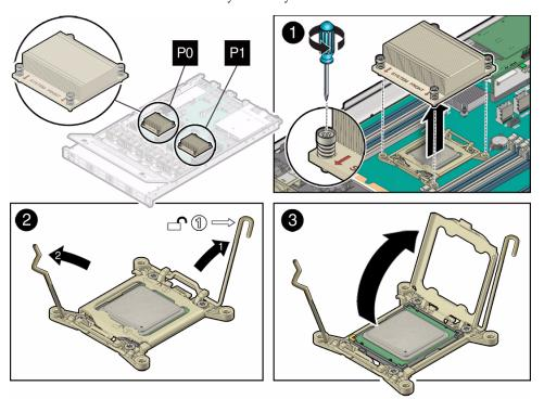
4. To separate the heatsink from the top of the processor, gently twist the heatsink left and right, while pulling upward, and then lift off the heatsink and place it upside down on a flat surface [1].
