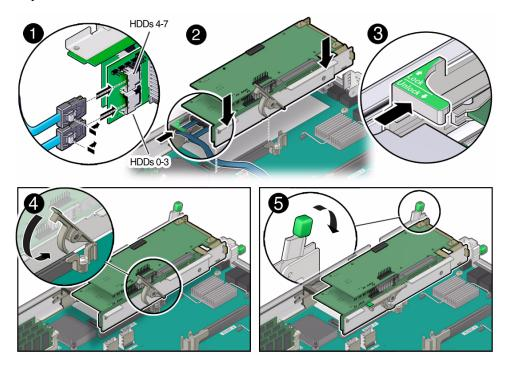
3. Raise the green-tabbed release lever on the PCIe riser to the open (up) position, and then gently press the riser into the motherboard connector until it is seated [2].
