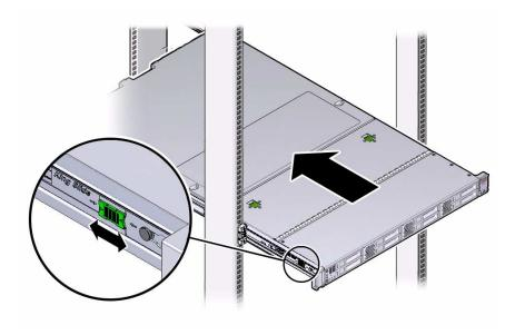
b. Continue pushing the server into the rack until the slide-rail locks (on the front of the server) engage the slide-rail assemblies.
