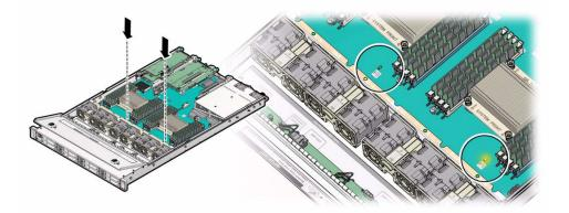
3. Gently press down on the top of the heatsink to counteract the pressure of the captive spring-loaded screws that secure the heatsink to the motherboard and loosen the four Phillips captive screws in the heatsink for the processor [1].
