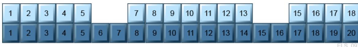
Figure 2–5 Dynamically Reclaimed Partitioned MVC
