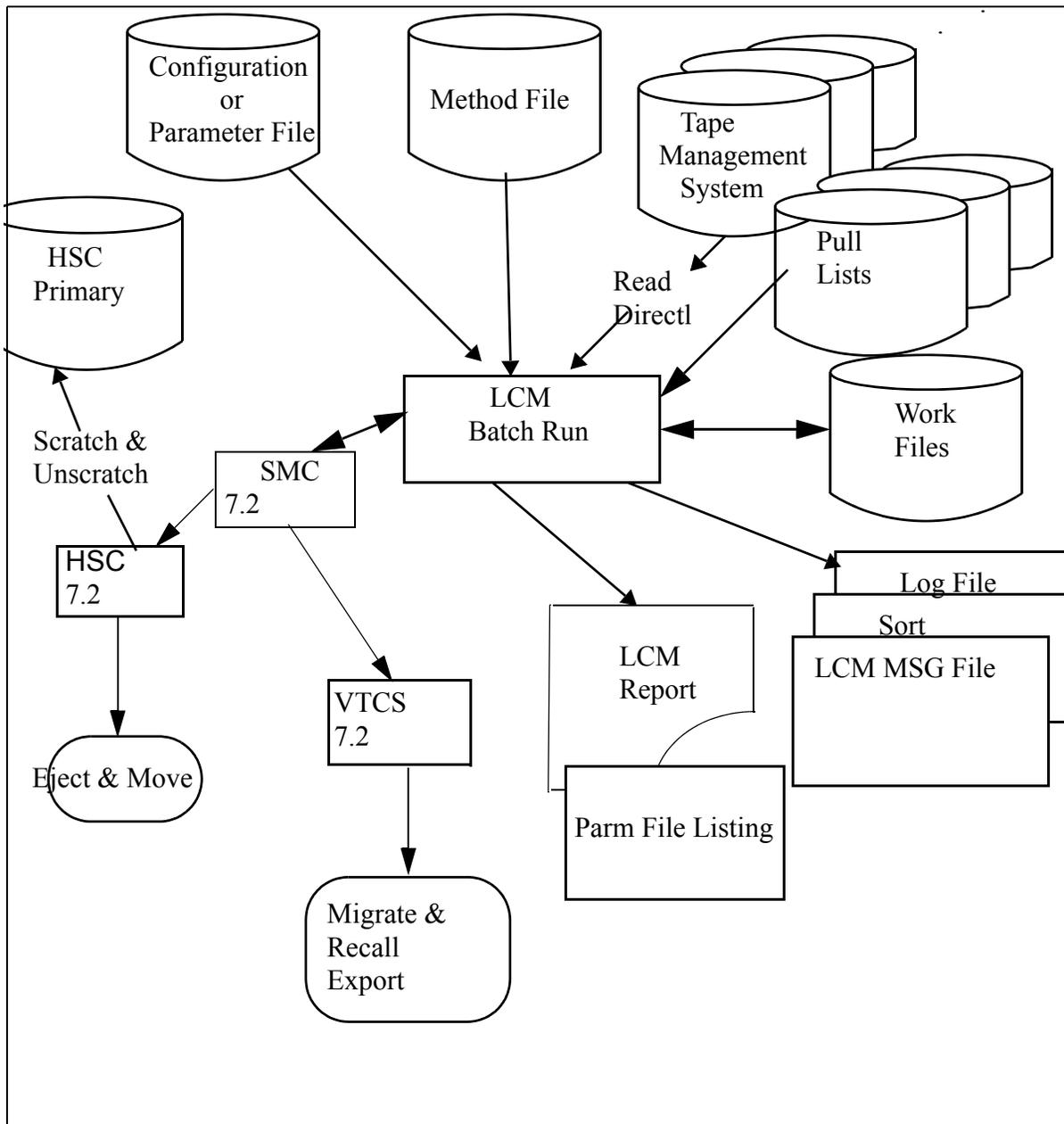
FIGURE 1-1 LCM Processing
