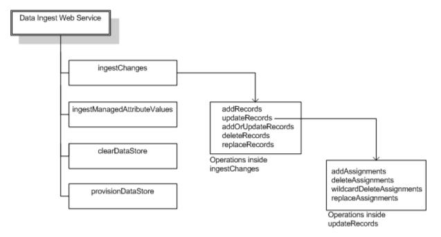
This diagram illustrates the Data Ingest Web Service structure:
