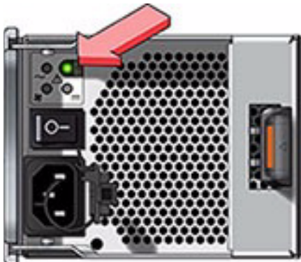
FIGURE: Disk Shelf Power Supply Status Indicator
