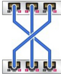
FIGURE: Connecting the Cluster Cables
