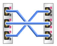
The ZS3-4 and 7x20 controllers provide three redundant links that enable the heads to communicate: two serial links (the outer two connectors) and an Ethernet link (the middle connector).
