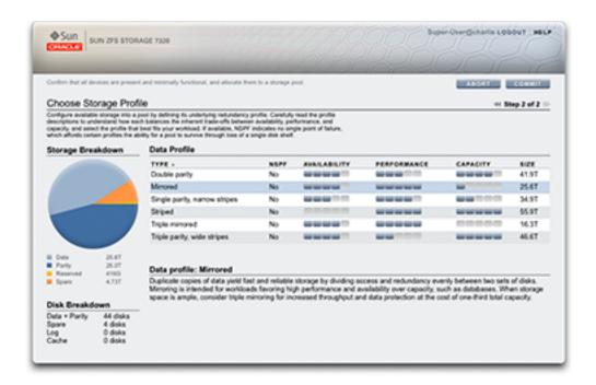
The ZFSSA Browser User Interface (BUI) is the graphical tool for administration of the appliance. The BUI provides an intuitive environment for administration tasks, visualizing concepts, and analyzing performance data. The BUI provides an uncluttered environment for visualizing system behavior and identifying performance issues with the appliance.
