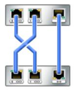
The ZS3-2 controller provides three redundant links that enable the heads to communicate: two serial links (the first two connectors) and an Ethernet link (the third connector).
