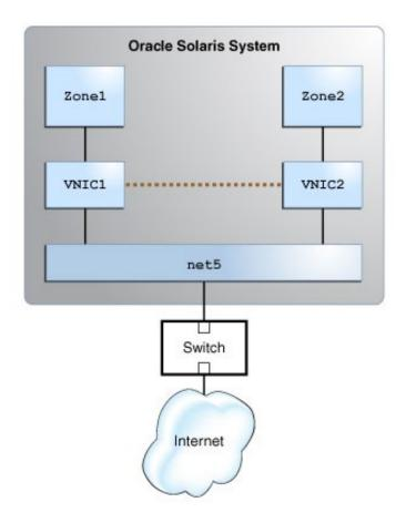
FIGURE 14 Internal Communication Between Zones
