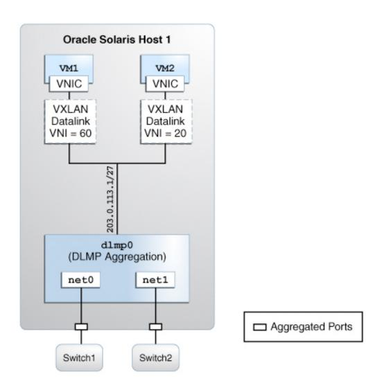
When an aggregated port or an external switch fails, VXLAN datalinks over the aggregation continue to exist as long as at least one port and a switch is functional, thereby providing
