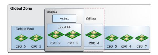
When you display datalink property information for pool and cpus, the EFFECTIVE column in the output shows the corresponding pool and CPU resources that are used for network processes, as shown in this example:
