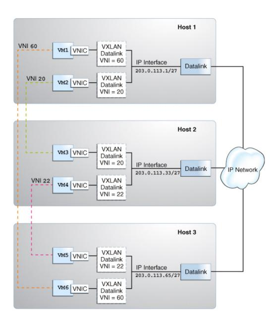
The figure shows three virtualized hosts attached to an IP network infrastructure. There are three VXLAN overlay networks identified by the VXLAN segment IDs or VNIs, 60, 20, and 22. The VMs VM1 and VM6 are on the overlay network identified by the VNI 60, the VMs VM2 and VM3 are on the overlay network identified by the VNI 20, and the VMs VM4 and VM5 are on the overlay network identified by the VNI 22.
