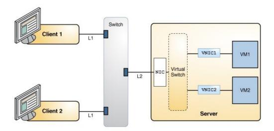
The following figure shows the same setup with EVB enabled:
