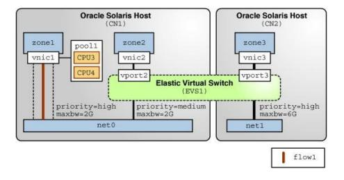
This figure shows the datalink and flow properties that are set for the VNICs and flow1. The following table describes these properties and their values.
