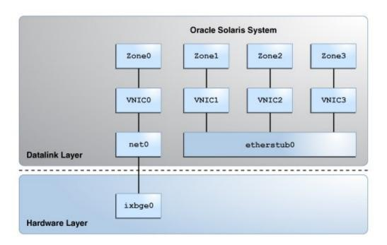
This figure shows etherstub0 over which VNIC1, VNIC2, and VNIC3 are configured. Each VNIC is assigned to a zone. The private virtual network based on the etherstub cannot be accessed by external networks. For more information, see "Use Case: Configuring a Private Virtual Network" on page 53.
