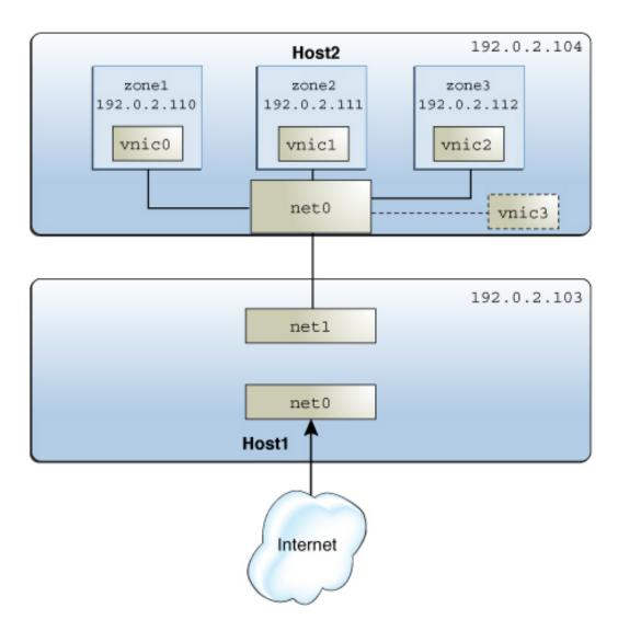
FIGURE 24 System Configuration for Managing Resources on Datalinks and Flows
