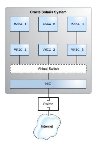
The figure shows a single system with one NIC. The NIC is configured with three VNICs. Each VNIC is assigned to a zone. The zones communicate with each other and with the external network by using their respective VNICs. The three VNICs connect to the underlying physical NIC through the virtual switch. The function of a virtual switch is equivalent to the function of a physical switch, which is to provide connectivity to the systems.
