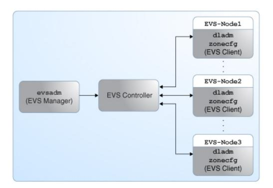
In this figure, the EVS manager and the EVS controller are two separate hosts. The EVS nodes EVS-Node1, EVS-Node2, and EVS-Node3 are three hosts whose VNICs or zone's VNIC anet resources connect to an elastic virtual switch.
