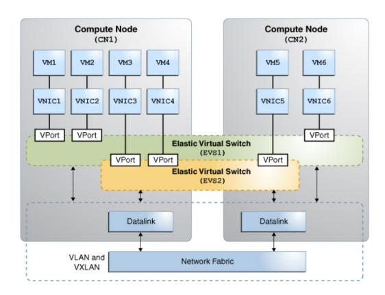
FIGURE 17 Elastic Virtual Switches Between Compute Nodes
